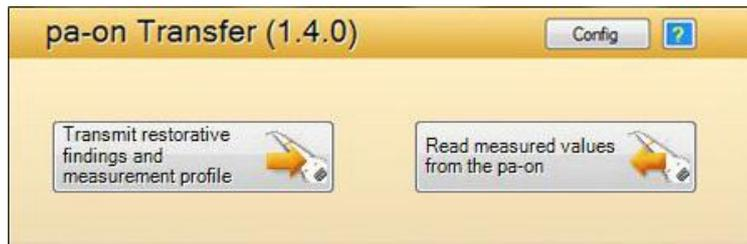
Before you can begin the measurement, you have to define where and what to measure. Therefore click on the button "Config" and choose a measuring profile. For details read the chapter "Configuration".
