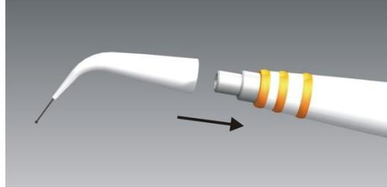
Calibrating the zero position: Gently push the thin metal probing needle into the plastic sheath until it stops. Be careful not to bend or twist the needle. This might happen on very smooth surfaces.
